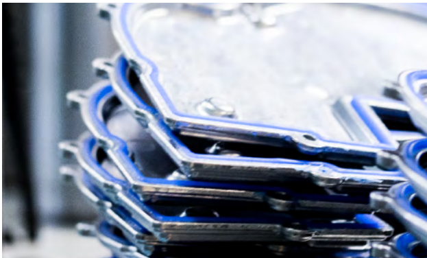
Pictured: Overmould of silicone on an Aluminium plate.
